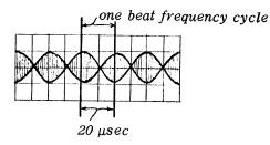
$180 \text{A} = 10 \, \text{mc}$  sine waves  $661 = .1 \, \mu \text{SEC/CYCLE}$  ( $10 \, \text{mc}$  sine waves) Test scope =  $10 \, \mu \text{sec/cm}$  Beat frequency =  $20 \, \mu \text{sec} = 50 \, \text{kc}$
