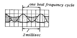
$180 \text{A} = 1 \, \mu \text{sec markers}$   $661 = 1 \, \mu \text{SEC/CYCLE}$  (1 mc sine waves) Test scope =  $500 \, \mu \text{sec/cm}$ Beat frequency = 2 millisec =  $500 \, \text{cps}$
